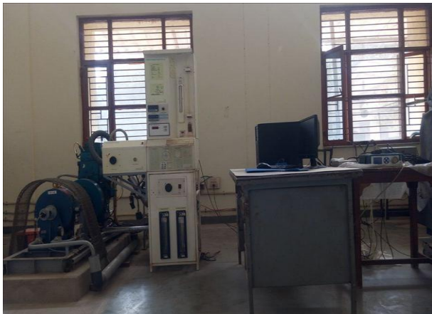
Figure 3.2 Computerized single cylinder diesel engine with smoke meter and gas analyser
